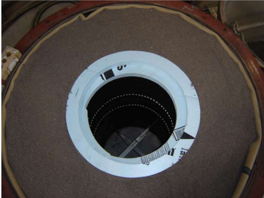
Figure 3: Plan view of Hoop Compression Cell with lid removed; under prep for profiled pipe test.
